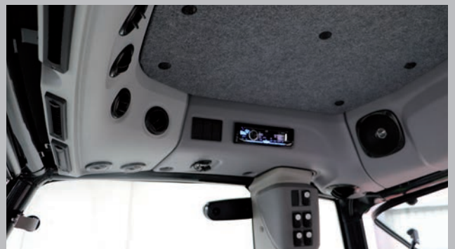
Air vents located throughout cabin.
